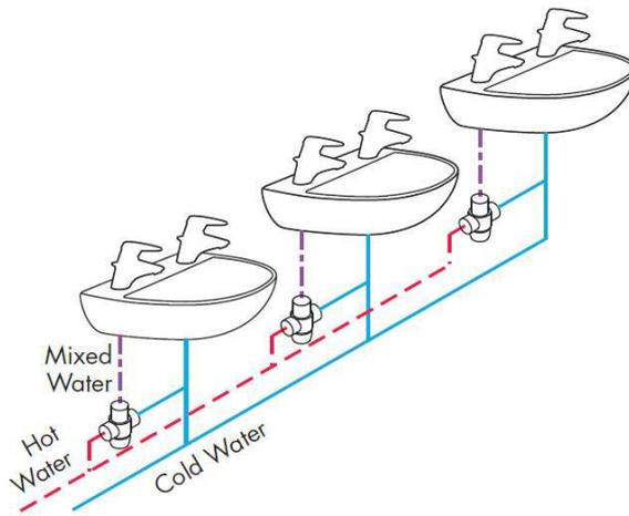
The HEAPE range of thermostatic mixing valves **MUST** be installed in an accessible position to ensure that maintenance,
