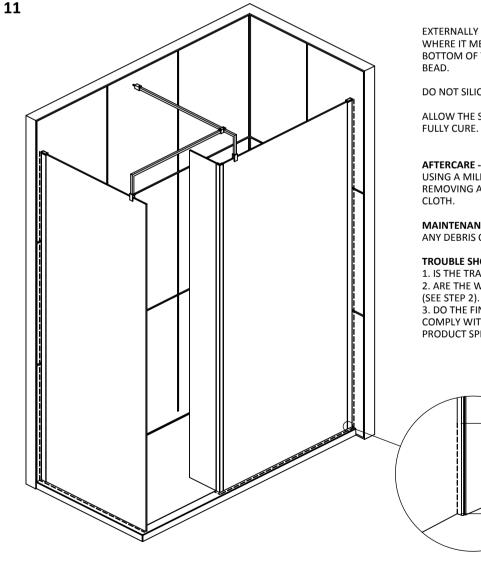
EXTERNALLY SILICONE SEAL THE WALL PROFILE WHERE IT MEETS THE WALL AND ALONG THE BOTTOM OF THE GLASS. ALL IN A CONTINUOUS
