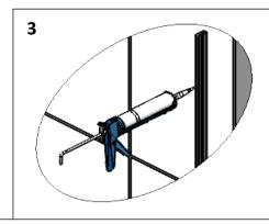
RUN A SMALL BEAD OF SILICONE DOWN THE INSIDE OF THE WALL PROFILES BEFORE FITTING GLASS. NOW SLIDE THE GLASS PANELS (ITEM 2) INTO THE PROFILES.
