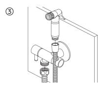
Attach the selected hose and shower handset to the bar valve. Turn on the mains water supply, check all joints/connections for any leaks.
