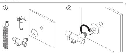
Make sure that all components are present prior to installation. Ensure the chosen wall selected has been prepared.
