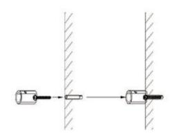
Step 2: Pinpoint the positions on the wall then drill Step 3: Connect the bracket socket to the wall with screws.
