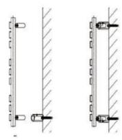
Step 5: Mount the towel rail to the wall and tighten the crews in the brackets.
