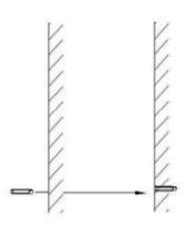
four holes accordingly and fix the wallplugs into the wall.
