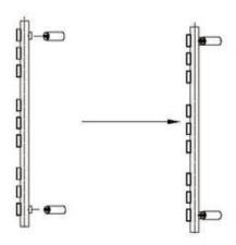
Step 4: Fix the brackets to the towel rail with screws.
