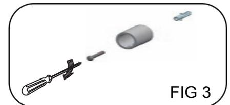
6. Insert rail into the wall bracket and tighten grub screws. Tighten glass bracket onto the glass.
