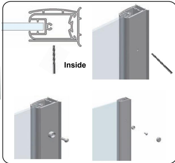
5. Insert the glass bracket **S033C** onto the long side of the rail and position towards the end of the glass panel. Insert the wall bracket **S035C** onto both ends of the rail. Level the rail and mark the fixing points to the wall.
