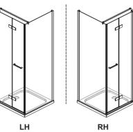
Note: Determine the handing, note that the wall profile is only fitted to the side panel.
