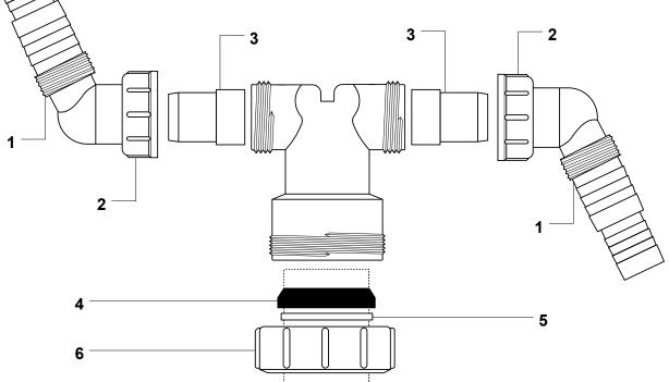
Multifit Outlet to suit 1.5" or 40mm Standpipe.
