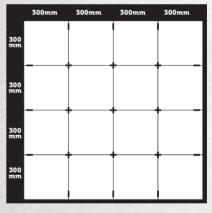
+ Spacer Bases can be used 1 per intersection, in place of 4 Straight Spacer Bases.
