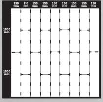
Straight Spacer Bases should also be used in straight grout joints, every 300mm from intersections.
