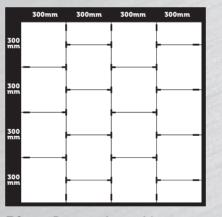
T Spacer Bases can be used 1 per intersection, in place of 3 Straight Spacer Bases.
