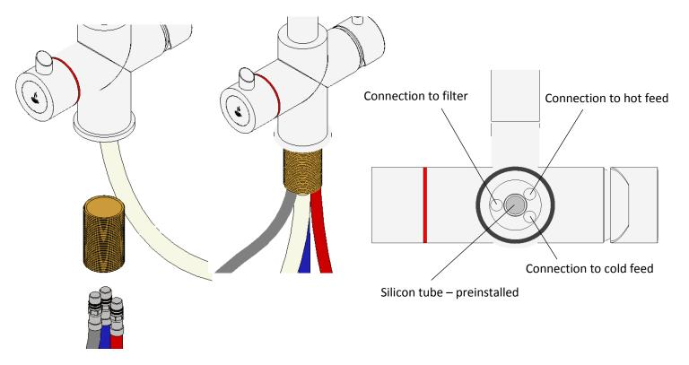
Feed the flexi tails through the mounting barrel and then hand tighten into the tap. Fit the tap in the desired location using the black plastic lock ring.
