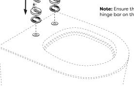
Once the hinge plates is fixed into position; place the cover caps over the hinge pins, then mount the toilet seat. Adjust the toilet seat to fit the pan.
