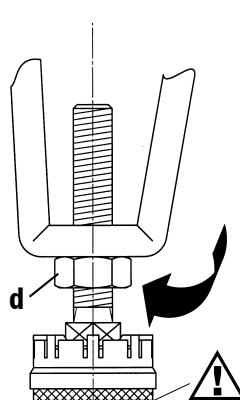
Turn over bath, align with the help of a spirit level by turning the screw and tighten the locknut (d). With the use of the Kaldewei sound insulation set, and provided installation is effected properly, the requirements of DIN 4109/A1 are fulfilled. Baths must also be mounted with bath anchors (not included in the scope of delivery)
