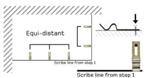
5. Turn the tray over and peel the protective film from the outer edges and waste only. Place the tray in situ and level both ways.
