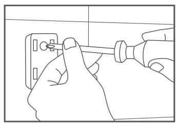
**4** Fix bracket into place using screws and fixings provided.
