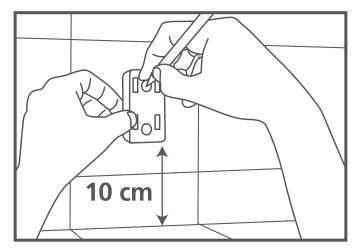
2 Lightly mark position of screw holes in bracket with a pencil.
