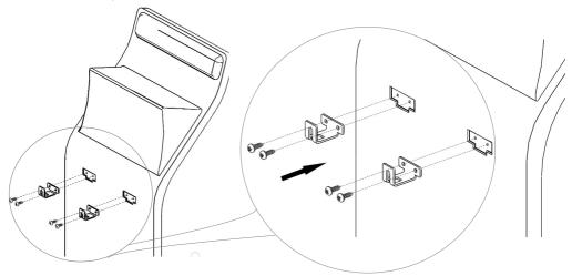
2 2 Attach the expansion anchors to the wall screws.
