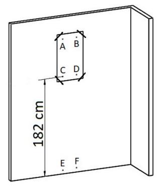
Bottom wall holes must be placed 182 cm from the floor.
