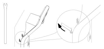
**2** 6 Tighten the column until it is completely secured and stable.
