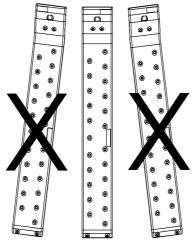
As for the lower fasteners, **mark** the wall with a pencil. **Remove** the column, drill two holes accordingly and insert the **wall plugs**.
