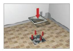
Place a small blob of tile adhesive in the middle of all four sides of the shower drain hole in the shower tray. Gently ease the shower drain top into position in the shower tray. Leave to set for approximately 3 to 5 hours
