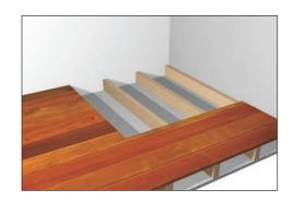
Before proceeding, check thoroughly for pipes and wires under the floor. Set the circular saw blade to the depth of the floor boards, it may be necessary to increase the depth slightly if it does not go right through the floor boards. As a safety precaution, we would recommend that the circular saw is plugged into an RCD protected socket. Using the circular saw, cut along the lines that you have marked and remove the flooring and all nails or screws.
