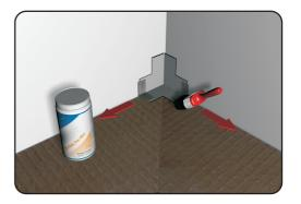
Put on the protective gloves and wear eye protection. Using the tape sealer and paint-brush, apply a thin layer of tape sealer to the internal corners of the shower area, slightly bigger than the pencil line marked in step 19.
