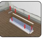
The linear drain is supplied with 2 No. square black plastic height adjustment nuts. Screw these on to the protruding bolts pre-fitted within the linear drain and adjust to suit your thickness of tile and adhesive. The drain should aim to be fitted flush with the finish tile.
