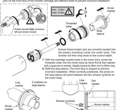
**IMPORTANT:** Before engaging the handle onto the diverter drive spindle, refit the plastic drive insert then: Align the dot marker on the handle with the line marker on the stop-sleeve. Reverse the sequence to refit the handle
