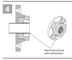
The pipes should be trimmed level to the wall bracket. If using a pipe cutter it will be necessary to mark the pipes and then remove the bracket before trimming to its correct length.
