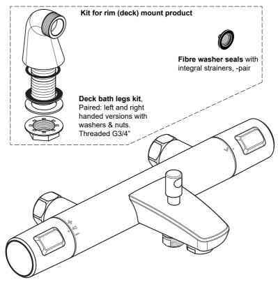
Deck bath/shower mixer shown without deck mounting legs assembled. Supplied with both A7207AA & A7698AA product. Right side handle controls flow. Diverter operates through the spout. Note: A7207AA is supplied without a shower kit, & A7698AA with supplied with the 600 riser rail & handset pack.
