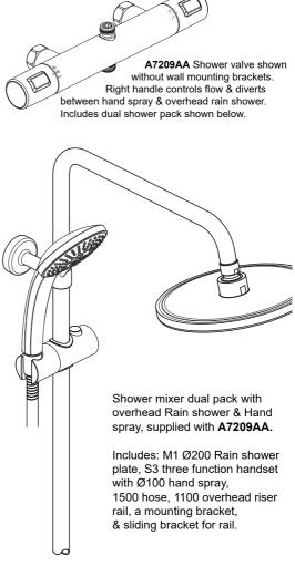
**NOTE:** Shower kits have to be carefully assembled during installation, chrome parts are packaged individually to prevent damage.
