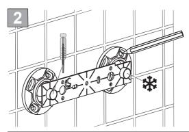
Place the brackets over the exposed pipes and use the template provided to position them 150mm apart.
