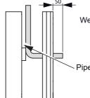
We recommend leaving 50mm of pipe protruding at this stage.
