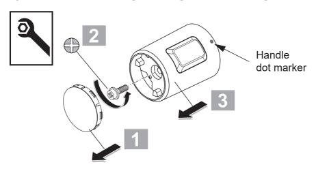
To gain access to either the thermostatic, flow or diverter cartridges, it will be necessary to remove the appropriate handle.
