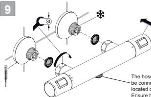
Assemble the shower valve to the adaptors remembering to ensure that the sealing washers or filters are inserted between the adaptors and the shower valve inlets.
