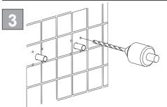
Drill holes appropriate for your choice of fixings into the wall.
