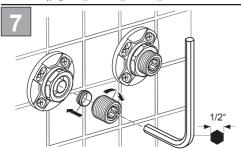
Fit the olives to the pipes prior to screwing the two 3/4" connectors into the wall mount plate using a 1/2" allen key. The connectors will have to be securely screwed in to form the necessary compression joint between the olive, wall plate and connector.
