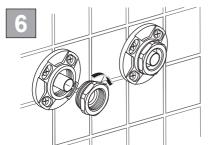
Screw the brass adaptors over the pipes into the plastic brackets. 36mm A/F Spanner flats are provided, hand tightness is adequate.
