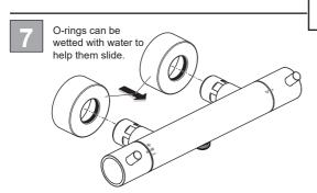
The two captive nuts should rotate freely.
