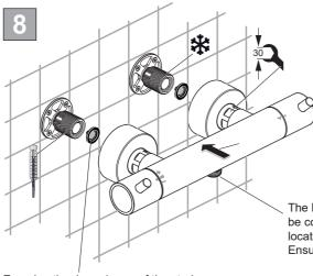
Assemble the shower mixer to the adaptors remembering to ensure that the sealing washers/ filters are inserted between the adaptors and the shower valve inlets. Keep the mixer parallel to the wall whilst screwing the captive nuts clockwise by hand. Carefully use a 30mm A/F spanner or strap wrench to tighten and make a water tight seal.
