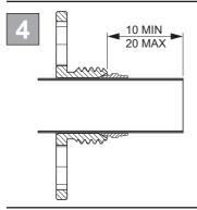
With the wall brackets in position, the supply pipes should be trimmed as shown. The pipes should project from the front face of the brackets by between 10 to 20mm.
