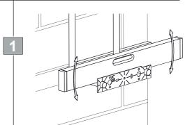
Ø15mm copper supply pipes should be run within the wall cavity. Hot supply pipe should be on the left hand side and the cold on the right.
