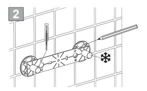
Place the brackets over the exposed pipes and use the template provided to position them 150mm apart.
