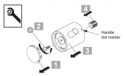
To gain access to either the thermostatic, flow or diverter cartridges, it will be necessary to remove the appropriate handle.
