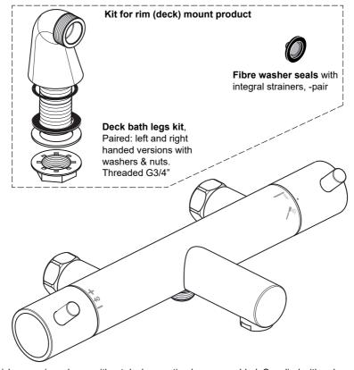
Deck bath/shower mixer shown without deck mounting legs assembled. Supplied with only **A7593AA** product. Right side handle controls flow & diverts between bath fill & shower hand set. Note: **A7593AA** is supplied without a shower kit.
