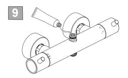
Note: the mixer supplied with A7594AA is fitted with an additional outlet nipple on the top surface to connect the over head shower plate.
