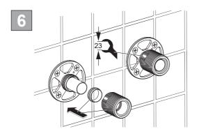
Slide the olives onto the pipes. Screw the two connectors onto the wall brackets by hand until they stop against the olives.
