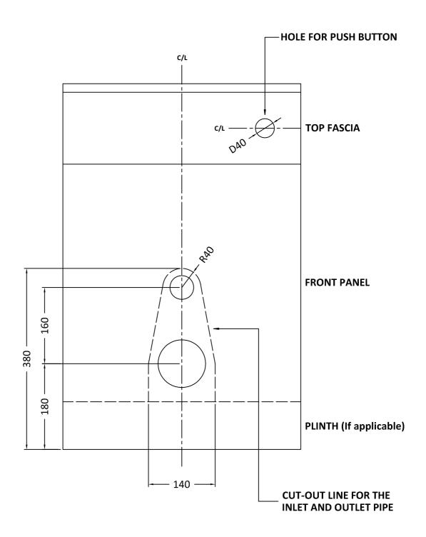
MARK OUT THE OPENING ON THE FRONT PANEL FOR THE INLET AND OUTLETS OF THE W.C. PAN. FOLLOWING THE ABOVE DIMENSIONS, CHECK THE SIZE AGAINST THE PAN BEFORE CUTTING OUT. DO NOT CUT OUT THE BOTTOM PLINTH!
