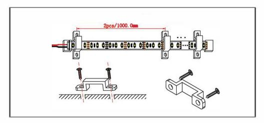
Using the rubber clips and screws that are supplied with this flexible strip, fix the strip to the desired location, as shown in the diagram above. Then connect the strip to the 15W IP44 rated driver (SE40560). Further instructions for the 15W IP44 rated driver are included in the driver pack.
