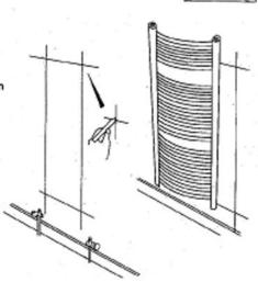
Mounting to Brick or Breezeblock At the required fixing positions drill hole using 8mm masonry bit and insert the wall plug E into the hole ensuring it's flush with the wall. Place long screw F through the centre of the wall support D and tighten into the wall plug.
