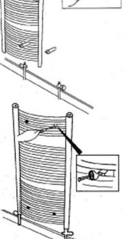
8 • Push the rail flat against the wall, adjust to required depth and tighten the small screws to secure. Push the end caps I over each of the bracket heads until they click into position.
