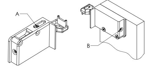
You may need to increase the length of the hook's protrusion. To do so turn screw 'B' anti-clockwise.
