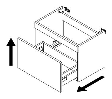
Remove drawer from cabinet prior to fixing unit to the wall. To do so pull-out the drawer to its full extension and gently lift the drawer box upwards.
