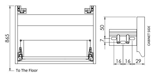
Fix Wall Hanging Plates as shown above. Check the type of wall you are fixing to and use the suitable fixings. (Not supplied).
