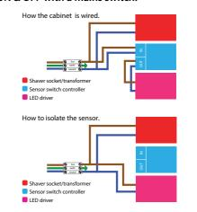
Re-wire the cabinet as shown in the diagram above. HiB recommends that all electrical bathroom products should only be fitted by a suitably qualified, Part P registered electrician.
