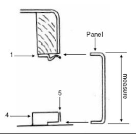
Note: It is also possible to secure the bottom of the panel using screws and plastic caps (not supplied)
