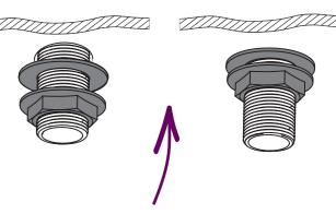
Secure the taps to the basin by using the washer and metal backnut below the basin.
