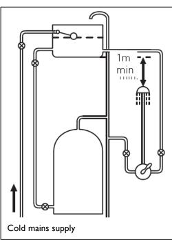
Important: If you install this shower valve with a gravity fed system, there must be a minimum head (vertical distance) from the underside of the cold water storage tank to the showerhead position of at least I metre.
