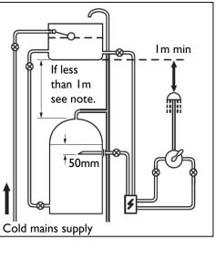
These fittings need to be installed in accordance with the following Installation Requirements and Notes (IRN) to ensure they meet the requirements of the Water Supply (Water Fittings) Regulations 1999 and the Scottish Byelaws 2004.
