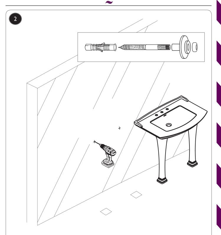
Drill the wall holes with an appropriate drill size, depending on the surfaces you are drilling into. If you are using wall plugs then insert them into the wall holes. The arrangement of the wall fixing bolts can be seen in the inset above.
