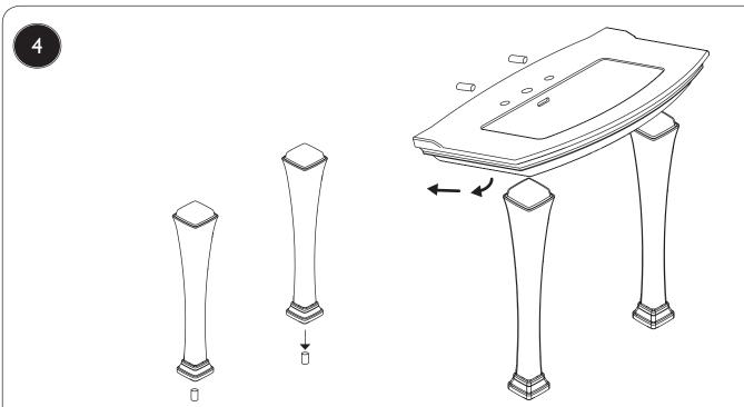
Seat the legs on the floor pins and and put the foam pad on top on the legs before you swivel the basin in by tilting the back onto the wall studs and lowering the front onto the legs. Finally, place the nylon washer and nut on the wall studs from underneath and tighten to secure the basin to the wall.
