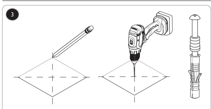
Use the foot print tracing to define the centre and drill an appropriate sized hole depending on the fixings used to secure the floor pins. Secure the fixing to the floor using the screw provided as per the illustration.
