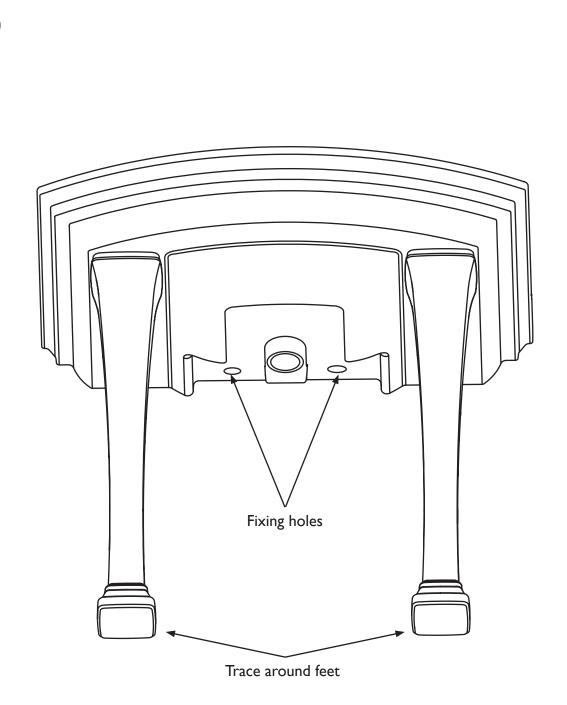
Rest the basin on the legs and butt up against the wall in the desired position and adjust using a spirit level till the basin is level. Mark the wall fixings holes located on the underneath rear of the basin and trace around the feet very lightly with a pencil. With the fixing holes and foot print outline marked, carefully place the basin aside.
