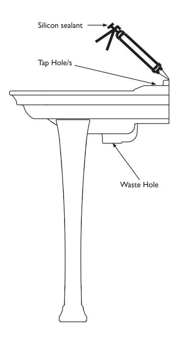
Fit the waste and taps to the basin (see separate fitting instructions) and seal around the back of the basin using appropriate coloured silicon sealant.
