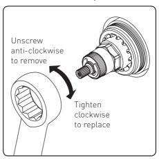
3. Remove the piston and thermostat assembly and place into a bowl.
