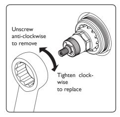
3. Remove the piston and thermostat assembly and place into a bowl. Carefully add hot water (just off the boil) and vinegar to de-scale. Leave in the solution until the water has cooled and rinse with clean water.
