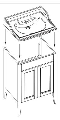
Locate the basin so it is evenly flush with the edges and firmly against the rear wall. Fasten basin to the wall using screws (not supplied) or bolts (supplied, if applicable). The holes for these can be seen on the rear of the basin.
