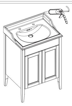
Once basin is fixed to the wall, run a bead of silicon around the joint between the basin and the vanity unit, this will ensure the furniture is sealed from water. Handles should be fitted by referring to accompanying instructions.
