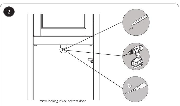
Mark the required hole using the bracket hole as a template. Drill a suitable hole for the wall fixings used (not supplied). Attach the bracket to the wall.
