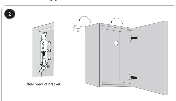
The hanging brackets are already secured to the cabinet, so you are able to hang cabinet in position on wall plates by adjusting the plate to allow enough of the hanger to protrude and hook onto the plate.
