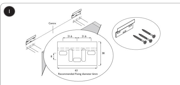
Determine favoured position of cabinet and mark a vertical centre point on the wall. Measure the span of the pre-fitted brackets and transfer measurement to wall measurement out from centre point to give a central position for the cabinet. Fit the wall plates using appropriate fixings (not supplied) using a long spirit level to make sure levelling is accurate. Plates should be no more wide apart than the spanned measurement of the wall hanging brackets.
