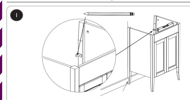
We recommend that you secure the unit to the wall using angled brackets (not supplied). Position the cabinet in your required location checking the alignment with a spirit level and mark the wall through the holes in the angled brackets. Make sure you removed required skirting boards before fixing. It is best to install the angled brackets on the inside of the freestanding furniture.
