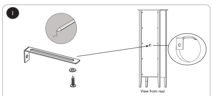
Tall boy units can be attached to the wall using the shown security bracket. There is a purpose access hole drilled for this on the lower part of the unit, use the provided screw and washer to attach the bracket to the unit.
