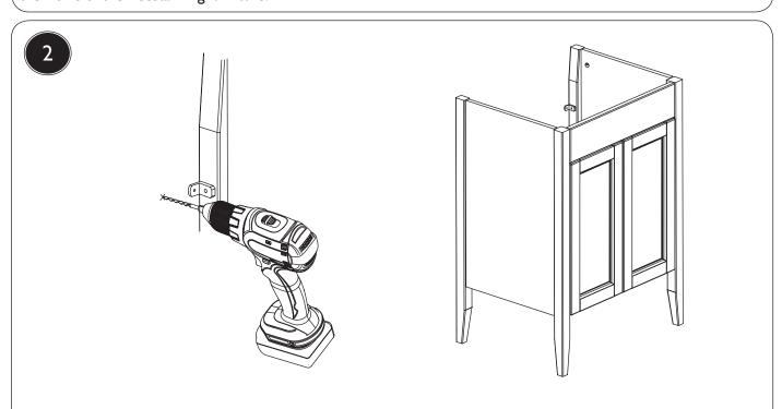
Remove the cabinet and drill holes of the appropriate size to accept the necessary screws or wall plugs used to secure. Lift the cabinet back into position and screw to the wall.
