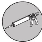
An additional bead of silicone sealant should be applied around the edge of the basin to prevent water ingress. Once cured, turn on the water supply to check all joints and connections for any leaks.
