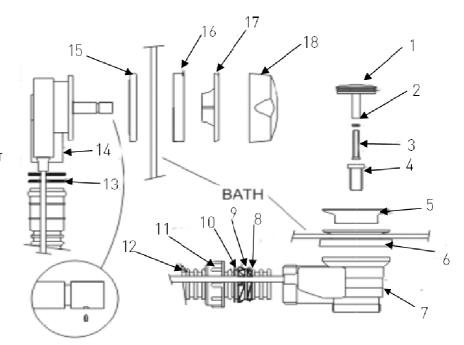
PLEASE NOTE: DO NOT PUSH THE HANDLE (18) ONTO THE SPINDLE (RINGED) OF THE OVERFLOW ELBOW (14), AS THIS WILL STOP WATER COMING OUT OF THE OVERFLOW. THERE IS A GRUB SCREW IN THE HANDLE THAT WILL LOCATE IN A HOLE ON THE SPINDLE.
