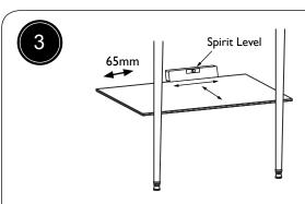
Carefully rest the glass shelf on the shelf rests and using a spirit level to level the glass shelf up horizontally at the back, and also from back to front, mark the wall from the top and bottom of the shelf around 65mm inwards from the sides of the glass shelf.
