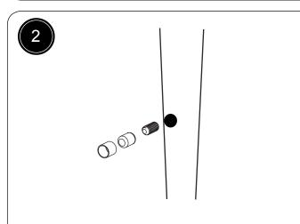
Insert the shelf rests into the holes at the back of the two legs.
