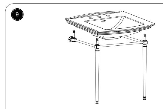
Locate the basin on the four chrome columns. If the product is supplied with inserts as seen in section 10, bear in mind that these need to be installed before levelling the basin.
