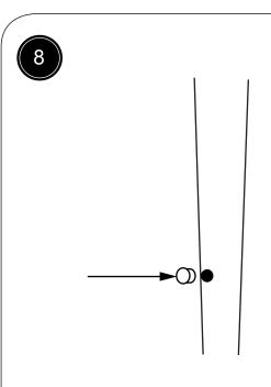
If the glass shelf is not going to be installed then use the 6 blanking plugs to cover the holes on the washstand.
