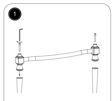
Attach both leg assemblies to the bottom of the front pole assemblies by using the M6 (35mm) hex bolt to secure the parts together.
