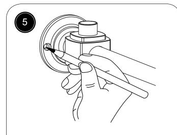
Locate the washstand on the newly installed Foot Stops and mark the location for the holes in the wall by using the washstand holes as the template. Ensure the washstand is level using a spirit level. Move the wash stand out of the way and Drill suitable holes.
