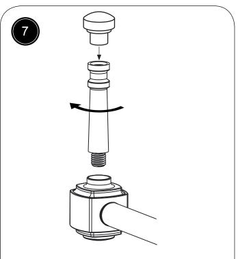
With the washstand in the correct position, add the chrome columns to the stand. Add the Basin Rests to the top of the chrome columns.
