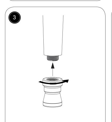
Attach the washstand feet to the base of the leg assemblies.
