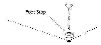
Using the dimensions (b & c) based on your washstand (page 5), accurately measure, mark and drill the holes in the floor for the foot stops and secure them down using the screws and suitable fixings for floor type.
