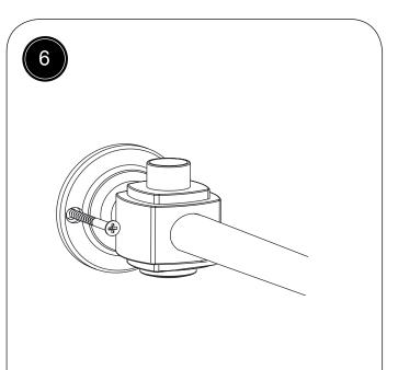
Secure the wash stand to the wall using suitable screws and wall plugs, depending on the wall type.
