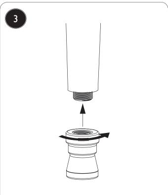
Attach the washstand feet to the base of the leg assemblies.
