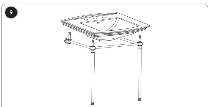
Locate the basin on the four chrome columns. If the product is supplied with inserts as seen in section 10, bear in mind that these need to be installed before levelling the basin.
