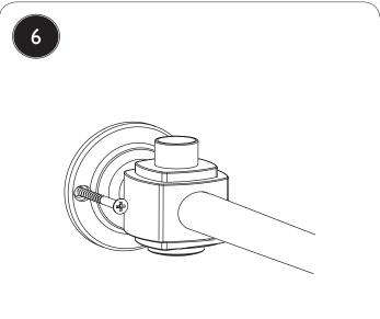
Secure the wash stand to the wall using suitable screws and wall plugs, depending on the wall type.
