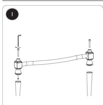
Attach both leg assemblies to the bottom of the front pole assemblies by using the M6 (35mm) hex bolt to secure the parts together.
