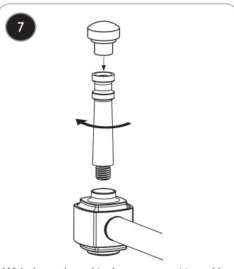
With the washstand in the correct position, add the chrome columns to the stand. Add the Basin Rests to the top of the chrome columns.
