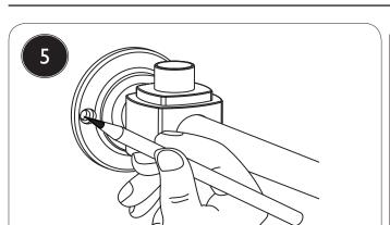
Locate the washstand on the newly installed Foot Stops and mark the location for the holes in the wall by using the washstand holes as the template. Ensure the washstand is level using a spirit level. Move the wash stand out of the way and Drill suitable holes.
