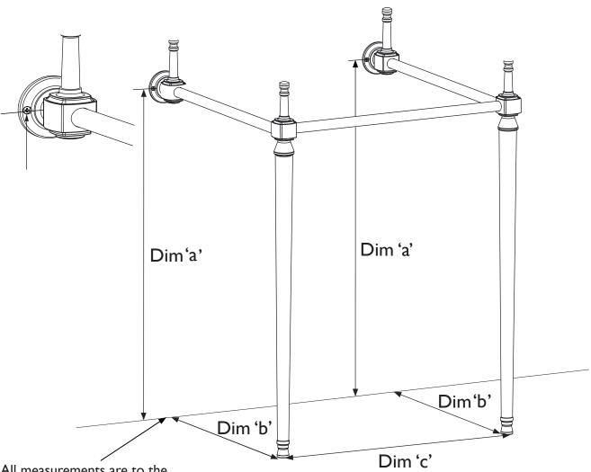
All measurements are to the centre of the legs, Dimension 'b' is measured to the wall and not the skirting board.
