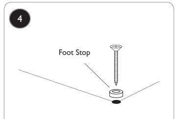
Using the dimensions (b & c) based on your washstand (page 5), accurately measure, mark and drill the holes in the floor for the foot stops and secure them down using the screws and suitable fixings for floor type.
