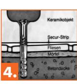
The balancing effect of the original-harosecur-Strip is shown in the graphics.
