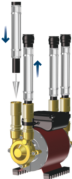
Fig. 17 Fitting the strainer basket
