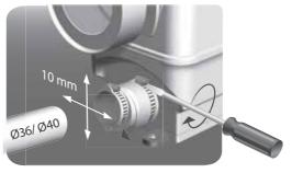
Fig. 35 Height and side alignment possible when using Ø40 inlet pipes
