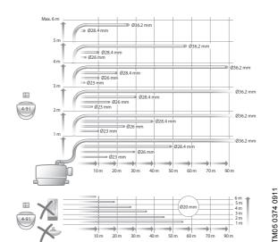
Fig. 13 Maximum lengths of vertical and horizontal discharge pipes
