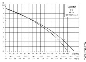
Fig. 36 Performance curves, Sololift2 C-3
