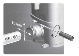
Fig. 17 Height and side alignment possible when using Ø40 inlet pipes
