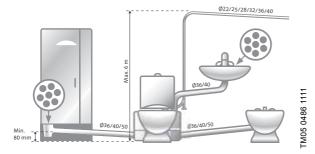
Fig. 14 Example of installation
