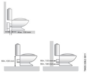
Fig. 7 Measurements to be observed
