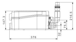
Fig. 44 Dimensional drawings, Sololift2 D-2
