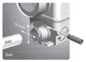
Fig. 25 Height and side alignment possible when using Ø40 inlet pipes
