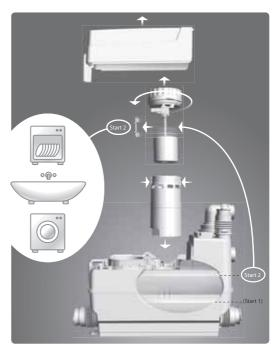
Fig. 33 Adjustment of the float switch
