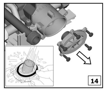
Remove the filter cap and flush with clean water and then replace.
