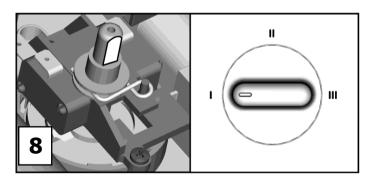
**Ensure** temperature Knob is aligned at 6 o'clock, whilst the 'spindle' in the product is rotated **fully** clockwise as shown **(fig.9)**.
