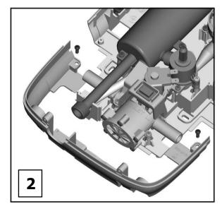
7. Decide the position of the electrical cable into the unit. Your shower offers the ability to have the connections on the right side or the left. (see fig.3).
