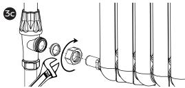
Feed the threaded tail nut through the inlet of vour chosen radiator. Secure the connection using an adjustable wrench
