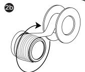
Unscrew the bottom compression nut and olive from the valve body. Slide the compression nut and olive over the metal pipe, then feed the metal pipe into the valve body. Secure the Piping to the valve body by screwing the bottom compression nut, tighten with a adjustable wrench.
