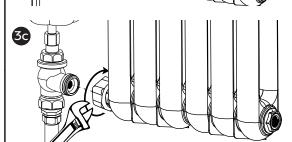
Feed the side union nut through the threaded tail, then screw the threaded tail to your chosen radiator. Secure the connection using an Allen key.
