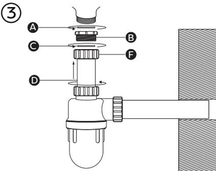
Place the 'Silicone O-ring' (A) over the threaded tail of the basin sink waste then screw the 'Top Screw Nut' (B) to the sink waste. Place the 'Silicone O-ring' (C) over the threaded tail of the 'Top Screw Nut' then slide the 'Body Tube' (D) upwards so that it reaches the sink waste and Tighten.
