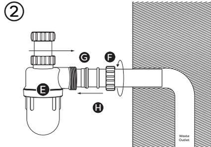
Place the 'Bottle Trap Body' (E) over the waste pipe, then fit the 'Silicone Seal' (G) and 'Plastic O-ring' (H) within the threaded tail. Screw the 'Body Nut' (F) to the 'Bottle Trap Body' ensuring a tight seal.
