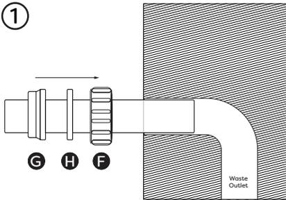
Place the 'Body Screw Nut' (F), 'Plastic O-ring' (H) and 'Silicone Seal' (G) over the waste pipe (not included) as shown in the diagram above.
