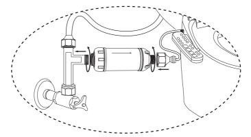
Screw the filter to the T-Valve connector (ensure that the arrow direction on the filter is pointing away from the T-Valve), then connect the PE inlet pipe to the other end of the filter. Turn on the water supply, check the connections for any leaks.
