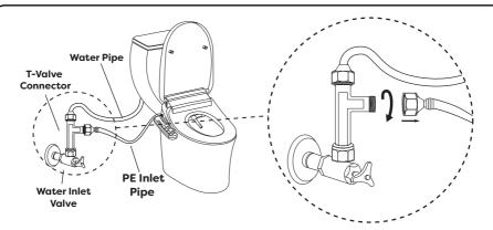
Unscrew the nut on the PE inlet pipe connecting to the T-Valve connector (as shown above). Make sure the water inlet valve is in the off position.
