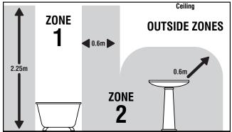
This product is suitable for use in Zone 2 and outside Zones of a bathroom. See diagram.
