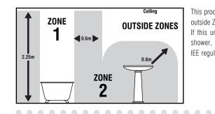
This product is IP44 rated, and is suitable for use in 1, 2 and outside Zones of a bathroom. See diagram. If this unit is being fitted in a room containing a bath or shower, a 30mA RCD must be used - in accordance with IEE regulations.
