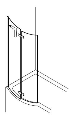
5.WITH THE HELP OF ANOTHER PERSON PLACE THE ASSEMBLED SCREEN INTO POSITION . MARK THE POSITIONS FOR THE 3 SIDE FIXINGS (SLIGHTLY OFFSET FROM THE WALL FIXINGS SO YOU CAN FIX THE COVER CAPS)ENSURE YOU DRILL THROUGH INTO THE FIRST PART OF THE HOLLOW BOX SECTION OF THE ALUMINIUM PROFILE ON THE FIXED SCREEN BEING CAREFUL NOT TO GO THROUGH THE OTHER SIDE( DO NOT DRILL INTO THE GLASS SECTION).DRILL THROUGH USING A 3.2 mm BIT AND FIX USING THE 10mm SELF TAPPING SCREWS.
