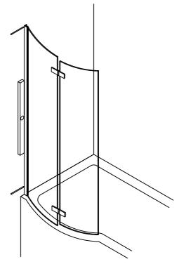
1. LAY THE FIXED AND HINGED PANEL CURVED FACE DOWN ON A PROTECTIVE SURFACE. DISASSEMBLE THE HINGES AND FIX TO THE PANELS AS SHOWN.
