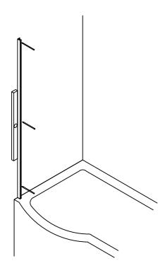
3. REMOVE THE SCREEN AND WALL POST FROM THE BATH, TAKE THE WALL POST AND PUT BACK INTO POSITION, USING A SPIRIT LEVEL TO ENSURE THAT THE POST IS PLUMB MARK THE POSITION OF THE 3 FIXING HOLES.
