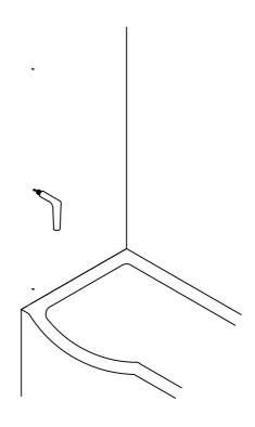
4. REMOVE THE WALL POST AND DRILL WHERE MARKED FOR THE WALL FIXINGS. REPLACE THE WALL POST AND SECURE INTO POSITION.
