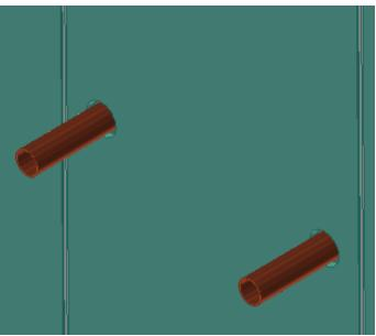
Ensure that your pipe centres are correct for your bar valve (usually 150mm) and ensure that your tiles / wall coverings are fully sealed and cured
