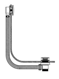
5. Tighten screw plastic nut to the waste body, and put back cover;
